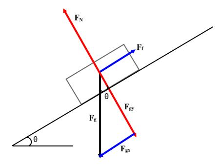
A worker places a large plastic waste container with a mass of 84 kg on the ramp of a loading dock as shown in the figure.
