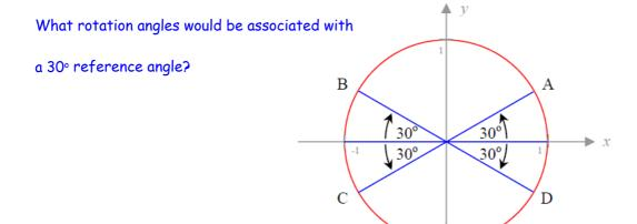
Determining rotation angle from a known reference angle ...
